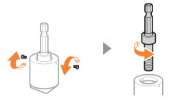
Remove the ring cover and then take out the disc spring and the washer.
