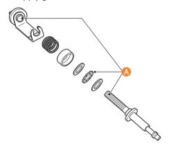
• Check whether the threaded shaft is bent or any foreign matter is adhered to it, and check whether the thread is worn.
