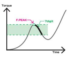
In the F. PEAK mode, the slip torque of the additional fastening is displayed. When the decreasing rate of the first peak down exceeds 7 digits, the maximum value at that point is displayed. Thereafter, the display does not change even if torque exceeding the maximum value is applied.
