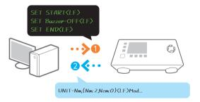
• Send a setting change command to the device. Send <SET START> and <SET END> before and after the setting change command.
