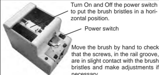
Move the brush by hand to check that the screws, in the rail groove, are in slight contact with the brush bristles and make adjustments if necessary.
