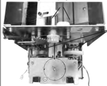
When the right pin is vertical, the left pin should be inclined about 46°.
