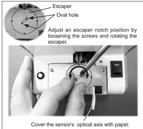
You can make fine adjustments for width clearance between the end of the rail and the escaper. Also, you can make fine adjustments for height clearance between the rail surface and the escaper surface.
