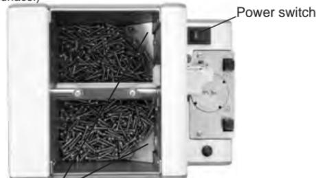
This inclined surface, on both the right and left inclined plates, should be visible.
