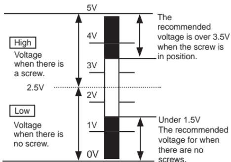
This is no malfunction when the voltage is slightly off of 2.5V. The adjustment, for ordinary screws, would be as described above. For screws which have a flatter head, refer to the figure on the left for adjustments. Depending on the screw-head height, it may be necessary to set the low-range voltage at more than 1.5V and the high-range voltage at under 3.5V.
