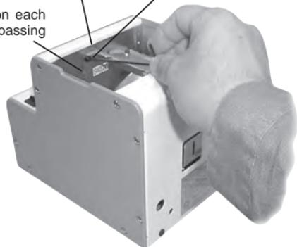
Remove the passing plate. Do not lose the attached bolts. Using bolts other than those supplied with this machine may result in a malfunction.
