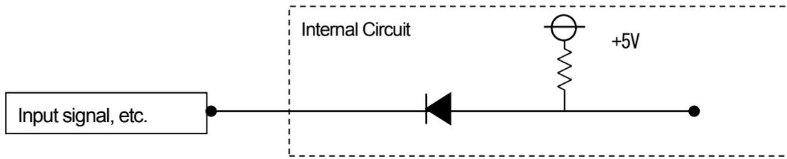
The reference structural outline when an external buzzer is installed and interlocks with the I/O BOX buzzer is externally installed (External power supply is needed for the external buzzer.)
