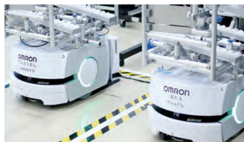
AMRs manufactured in-house transport finished products and supply empty boxes.
